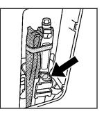
Install the jack in the left side panel of cargo area and secure with the wing bolt.
